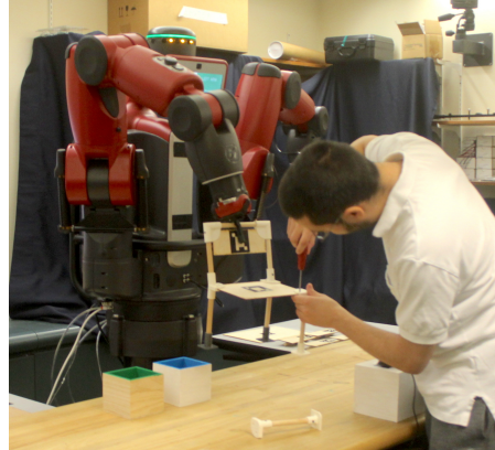
Fig. 1. Human participant engaged in the joint construction of a chair with the Baxter Research Robot. More precisely, the robot is providing support by holding the chair in place while the human partner is screwing a leg.
