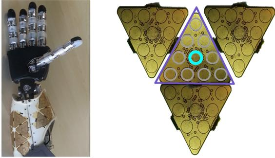
Fig. 2: *Pressure-sensitive skin of the iCub.* (left) iCub forearm with exposed skin patches. (right) Four triangular modules with 10 taxels each.
