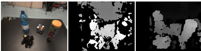
Fig. 2. Left: A typical scene seen by the robot. Middle: The depth map retrieved by the vision system based on pure kinematics calibration, producing poor results. Right: The improved depth map obtained after the calibration described in Section III-A.
